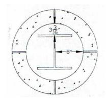
Steel Column - Minimum size W10x49 with minimum air space from web to block of 8 in. and from flange to block of 3 3/16 in. See above illustration.
